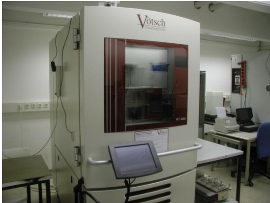
Fig. 10: Climatic chamber with control PC
