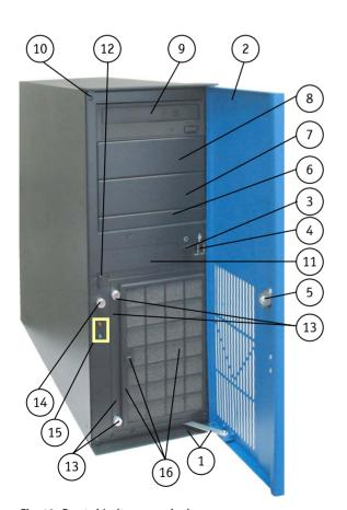
Fig. 13: Front side (tower version) with opened front access panel
