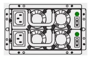
Fig. 20: Detail: 500W AC redundant wide range PSU
