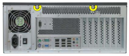
Fig. 29: Loosening the knurled screw on the rear side
