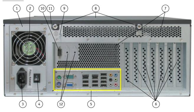
Fig. 16: Rear side of a KISS 4U V2 platform with motherboard and AC wide range PSU
