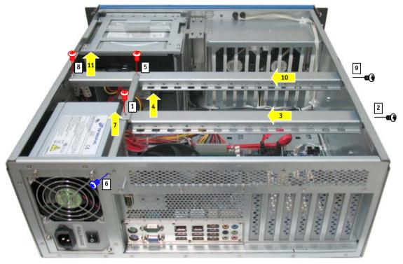
Fig. 34: Opened KISS 4U V2 platform - removing the card hold down brackets
