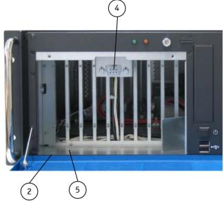
Fig. 46: Detail: Fan compartment (without fan slide-in module)
