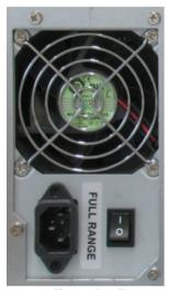
Fig. 18: Detail: 400W AC wide range PSU
