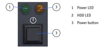
Fig. 9: Power button and LED indicators
