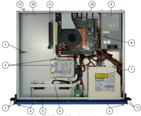
Fig. 5: KISS 1U Short V2 platform, rackmount version, opened
