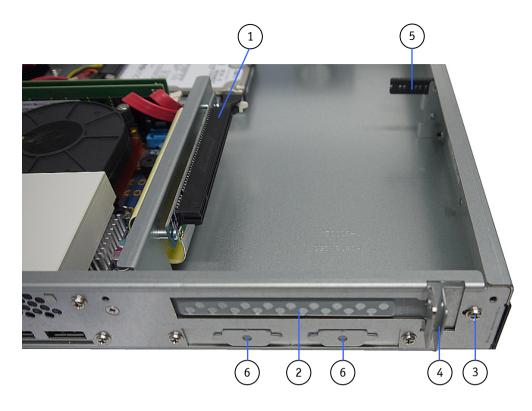
Fig. 19: Detail with opened slide bracket for PCI card slot
