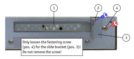
*Fig. 17: Detail: Rear side with slide bracket closed (for fixing the expansion card/slot bracket)*
