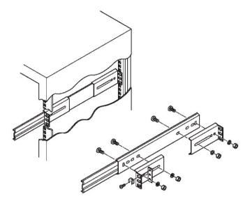
Fig. 28: Assembling the "Telescopic Rail" set
