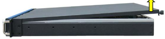
Fig. 16: Removing the cover
