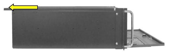
4. Lift the cover up (on the rear edge) and remove it (Figure 28).
