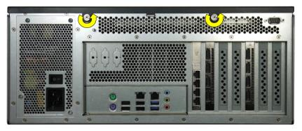
**3.** Pull the cover out a little bit (Figure 27) to release the cover fixing brackets (Figure 25, pos.3 and pos. 4) from the retaining plate of the chassis (see Figure 22, Figure 23, pos. 4) on the front side.
