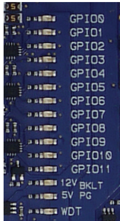
Figure 11: GPIO and Backlight LEDs, see board position 19
