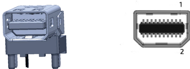
Figure 16: 20-pin eDP connector
