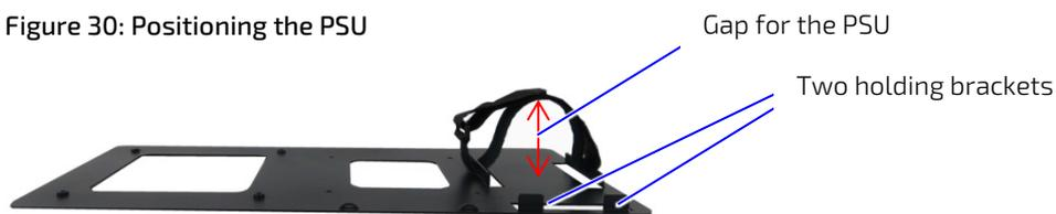
6. Slot the PSU, with the 3-pin AC connector facing towards the bottom of the VESA 100 mounting frame, into the gap made in step 5 and feed the PSU between the left and right PSU aligning brackets. Push down until the PSU rests on the two holding brackets at the bottom.
