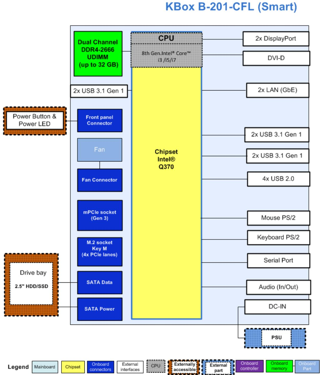
Figure 37: KBox B-201-CFL (Value) Block Diagram
