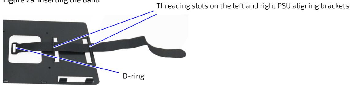
5. Double back with the flexible hook and loop band and feed the rough end through the band's D-ring. Pull the band through the D-ring and press approximately 30 mm to 50 mm of the self-gripping sides together to form a loose loop. Lift the bottom part of the loop to meet the top part to form a gap between the band and the VESA 100 mounting frame, as shown in Figure 30.
