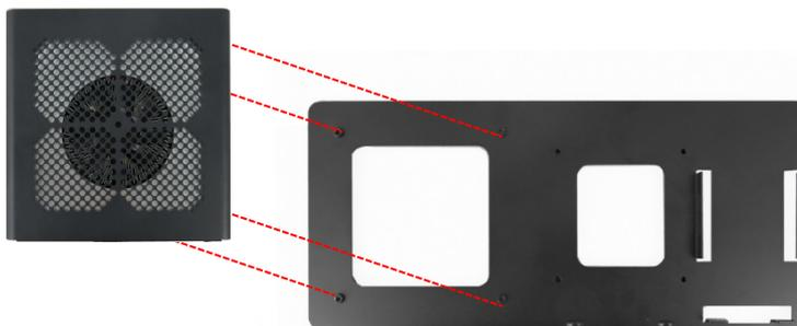
3. Insert the supplied four M3x 8 mm screws into the rear side of the VESA 100 mounting frame and using a Torx screwdriver (10) fasten the chassis to the VESA 100 mounting frame.
