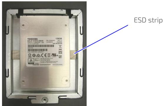
3. Align the SSD's connector with the internal SATA connector.
