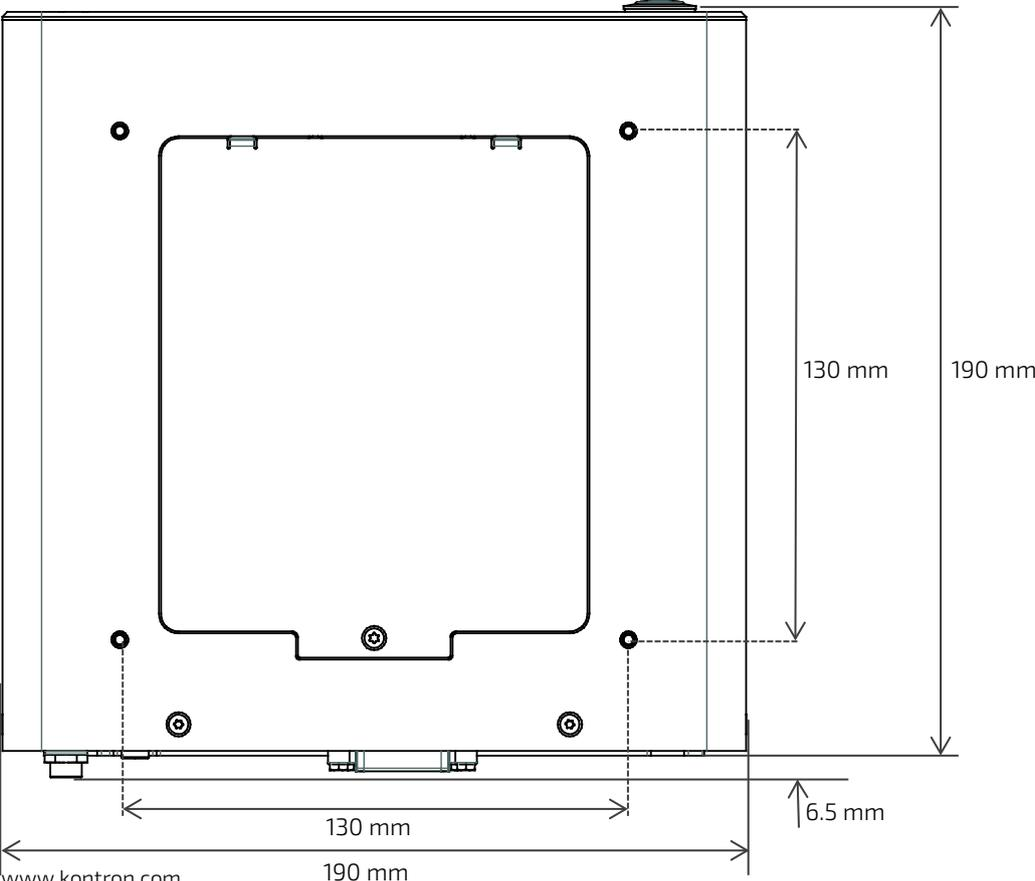
Figure 42: Dimensions Right Side and Left Side
