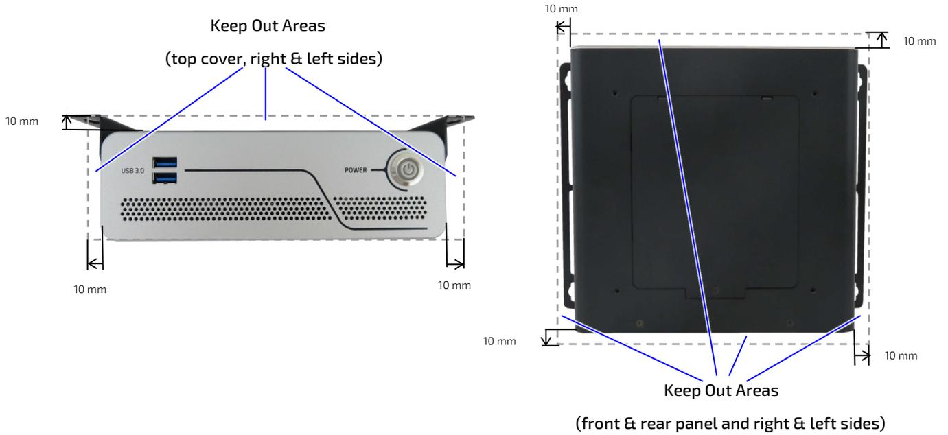
Figure 24: Keep Out Areas – with Bottom Side facing the Mount Surface
