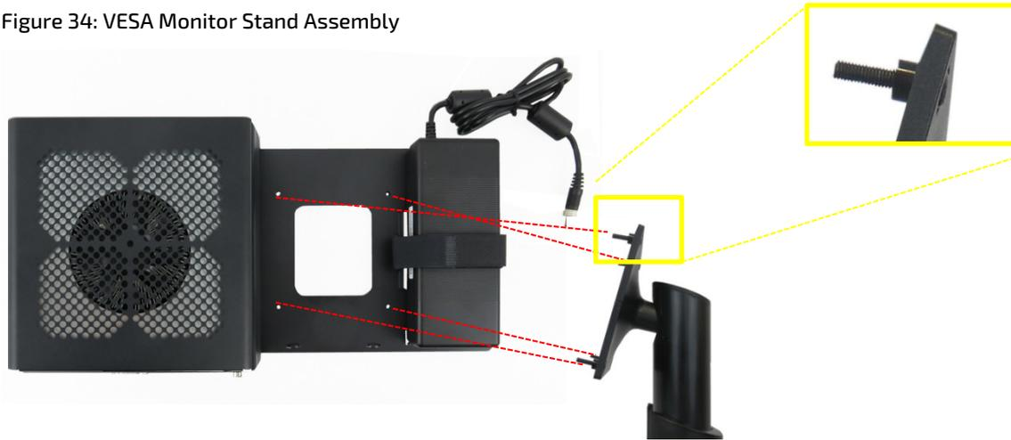
3. First insert the free end of the screw (with spacer) through the four mount hole on the VESA mount frame and then onto the VESA 100 mount hole on the back of the monitor.
