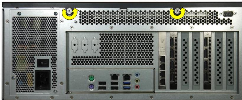
3. Pull the cover out a little bit (Figure 24) to release the cover fixing brackets (Figure 22, pos.3 and pos. 4) from the retaining plate of the chassis (see Figure 20, pos. 4) on the front side.
