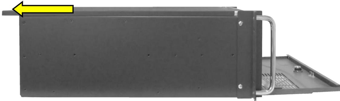
4. Lift the cover up (on the rear edge) and remove it (Figure 25).
