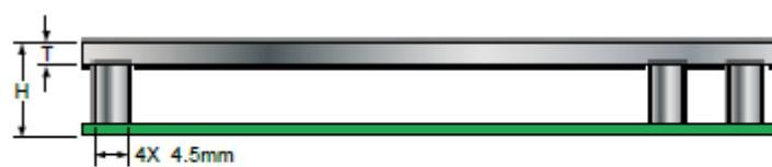
Cooling solutions provided from Kontron Europe GmbH for compact sized Computer-on-Modules are 27mm in height from module bottom to Heatsink top. Universal Cooling solutions to be mounted on the HSP (36099-0000-00-x) are 14.3mm in height for an overall height of 27.3mm from module bottom to Heatsink top.
