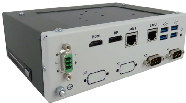
Figure 3: KBox A-150-SKL Chassis Variants
