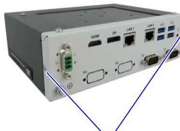
B) Remove front panel right and left side screws
