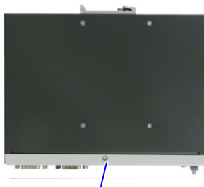
A) Remove front panel bottom side screw
