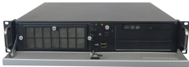
Figure 5: Rackmount variant (opened front access panel) Figure 6: Desktop variant (opened front access panel)
