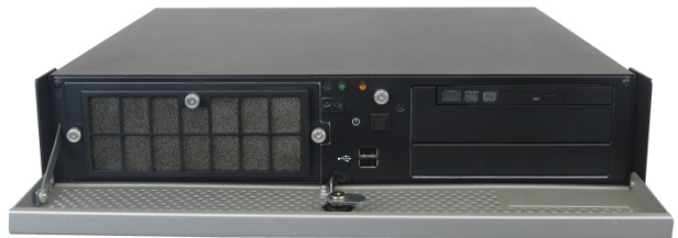
Figure 5: Rackmount variant (opened front access panel) Figure 6: Desktop variant (opened front access panel)
