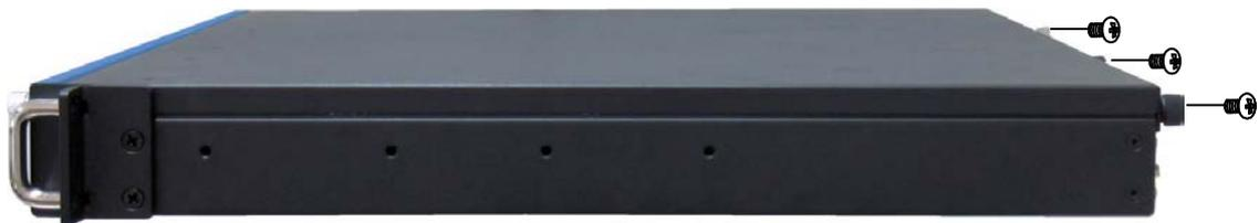
*Fig. 14: Loosening the three fastening screws on the rear side of the KISS 1U Short V2 system*
