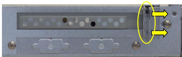
Fig. 18: Detail: Rear side with slide bracket (opened)
