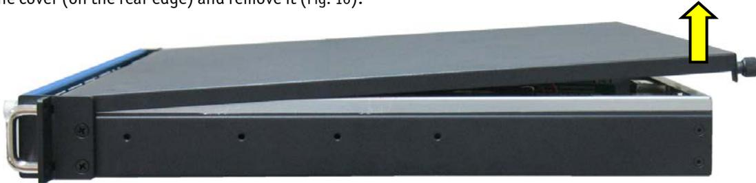
Fig. 16: Removing the cover
