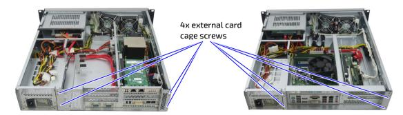
**6.** Install/remove the expansion card (/s) in/from the respective expansion slot (/s) and fasten the expansion card(/s) or the slot bracket(/s) to the card cage (Figure 23, Figure 24, pos. 9).
