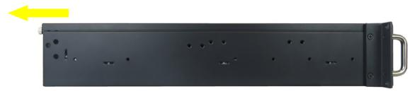
4. Lift the cover up (on the rear edge) and remove the cover as shown in Figure 29.
