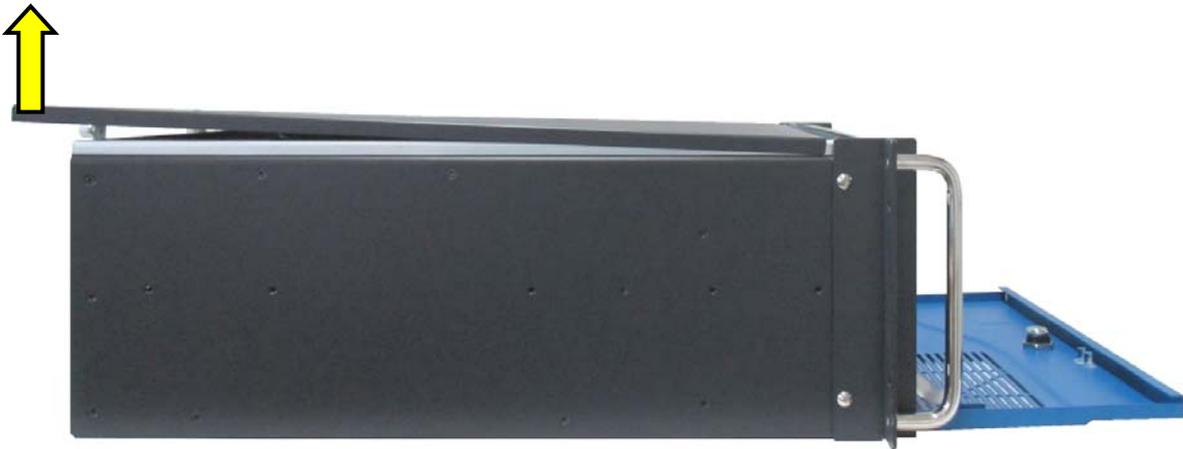
Fig. 31: Removing the cover
