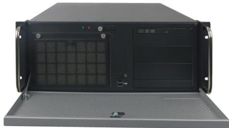
Figure 6: Desktop variant (opened front access panel)
