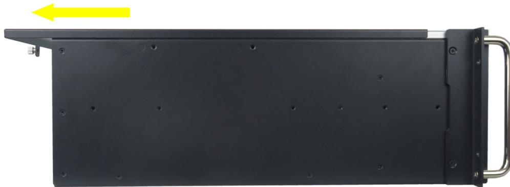
4. Lift the cover up (on the rear edge) and remove the cover as shown in Figure 29.
