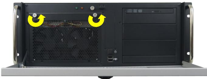
Figure 44: Fan compartment (without fan assembly)
