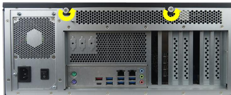
3. Pull the cover out slightly as shown in Figure 28 to release the cover's centering and fixing brackets (Figure 21, pos.3 and pos. 4) from the retaining brackets of the chassis (Figure 22, pos. 4).
