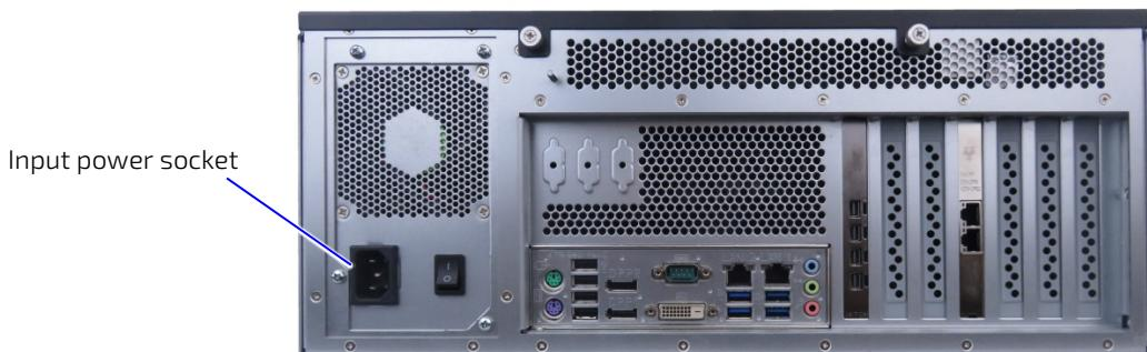
The input power socket is located on the rear side. To connect the power and start up, proceed as follows:
