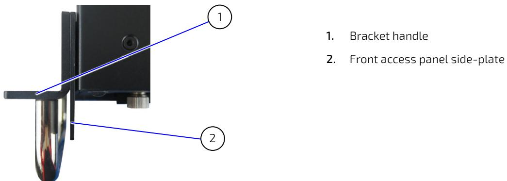
To remove the front access panel and front access side-plates, proceed as follows:
