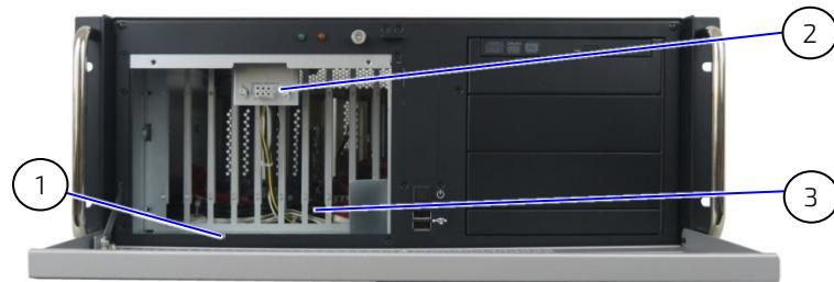
1. Fixing plate for the fan assembly
