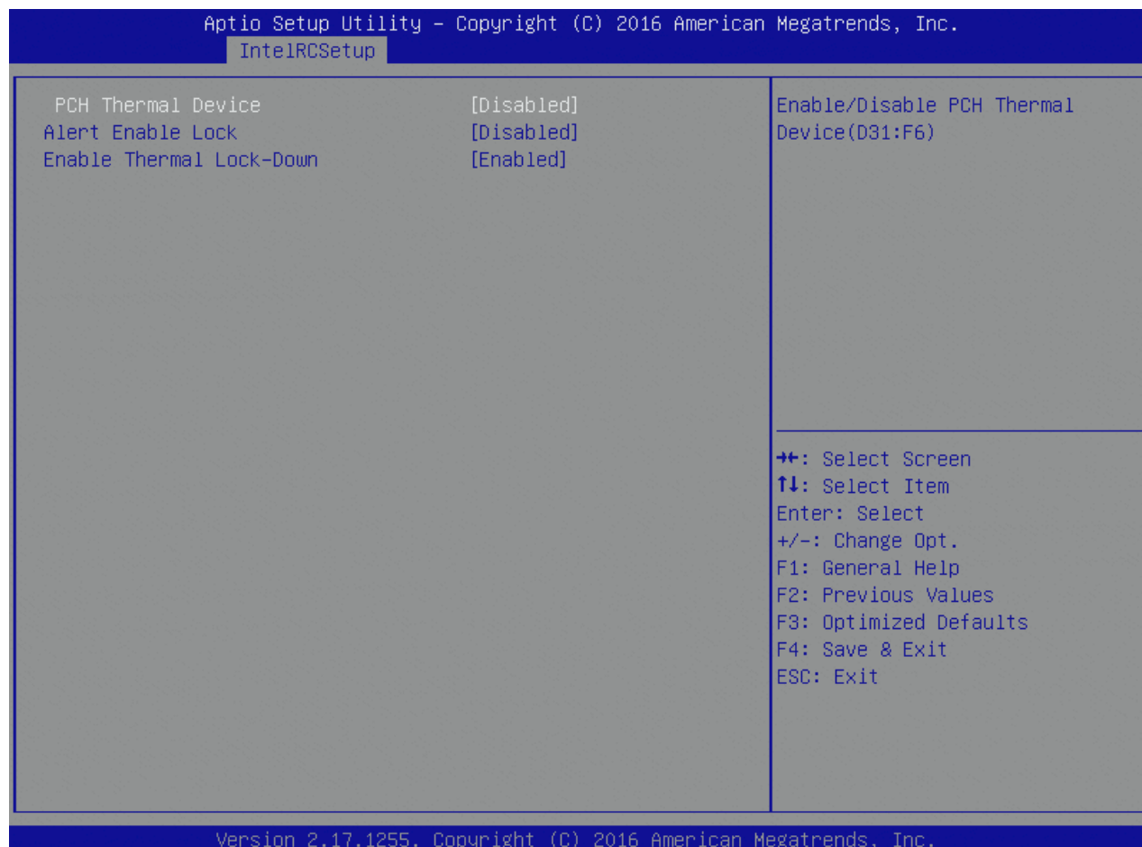
Figure 96: Platform Thermal Configuration Menu Screen
