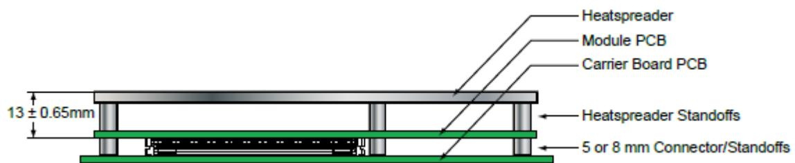
Cooling solutions provided from Kontron Europe GmbH for basic sized Computer-on-Modules are 27mm in height from module bottom to Heatsink top.
