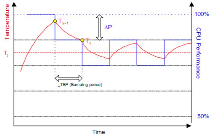
The ACPI OS assesses the optimum CPU performance change necessary to lower the temperature using the following equation
