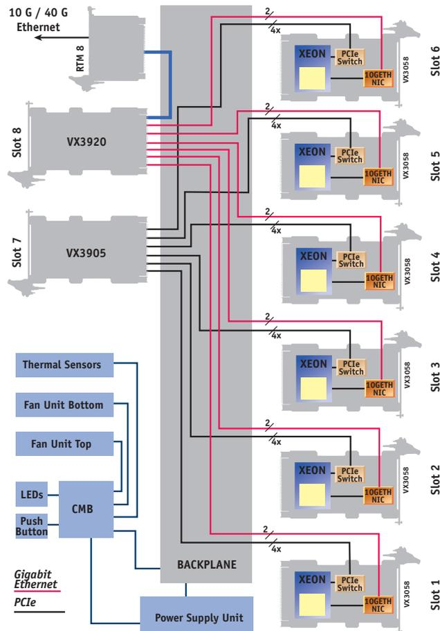
planes, for 10 GETH and for PCI Express, respectively. A unique API with TCP/IP sockets makes it a powerful, leading edge Multi-CPU computing node architecture.
