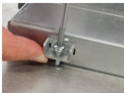
Figure 9: Fastening the Clamping Bracket
