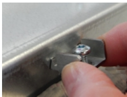
Figure 8: Clamping Bracket Insertion
