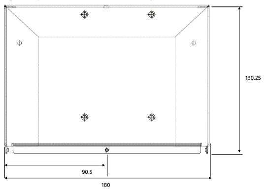
Figure 20: Side View Dimensions with HDD/SSD drive bay (Measurements in mm)
