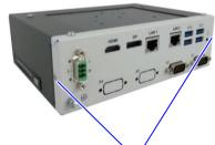
B) Remove front panel right and left side screws
