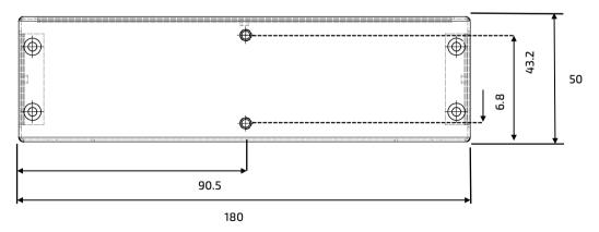
Figure 23: Top Side Dimensions without drive bay (Measurements in mm)
