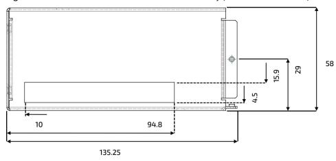
The following outline dimensions drawings shows the main external mechanical features for the KBoxA-150-BYT without an external HDD/SSD drive bay. All dimensions are shown in mm.
