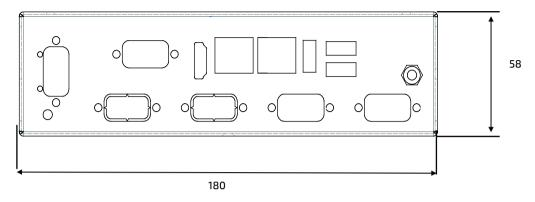
Figure 18: Rear Side Dimensions with HDD/SSD drive bay (Measurements in mm)
