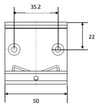
Clip the top of the DIN rail clamp in to the DIN rail and push the bottom of the DIN rail firmly until it clamps on to the bottom of the DIN rail.
