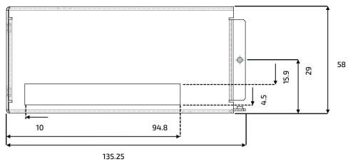
The following outline dimensions drawings shows the main external mechanical features for the KBoxA-150-BYT without an external HDD/SSD drive bay.
