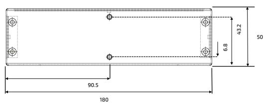
Figure 23: Top Side Dimensions without HDD/SSD Drive Bay (Measurements in mm)
