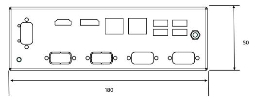
Figure 22: Rear Side Dimensions without HDD/SSD Drive Bay (Measurements in mm)
