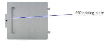
5. Slide the SSD drive bay cover forward slightly, to release the two aligning tabs (Figure 13).
