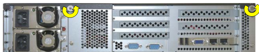
Fig. 26: Loosen the knurled screw on the rear side
