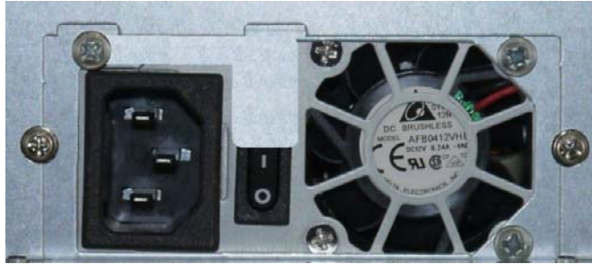
Fig. 18: Detail: AC Wide Rang PSU
