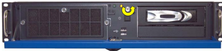
Fig. 25: Loosen the cover fastening knurled screw on the front side
