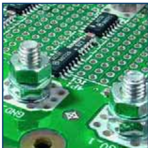
B - Power bolts M3/M4 cable lug (30 A/70 A)
