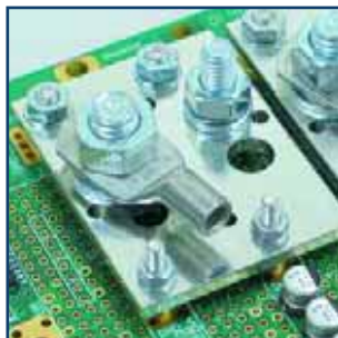
3 - Power plate (> 7 slot) M6/M8 cable lug (150 A)
