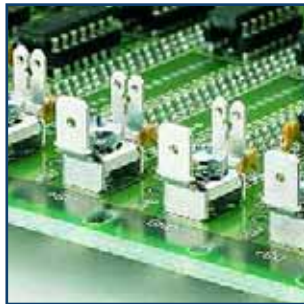
1 - Faston/M4 screw 2 x 6.3 x 0.8 (12 A)/ M4 cable lug (70 A)
