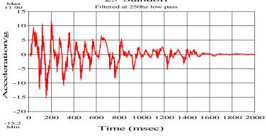
Accelerometer 7 on rack
