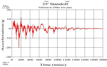
Accelerometer 11 close to Acc 7 but on server: High frequency spike due to slide bottoming is noted on first rebound (20g)
