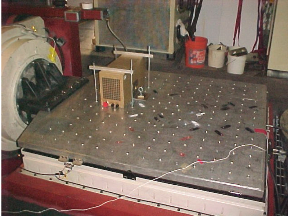
Figure 10: Transverse Vibration and Shock Test Setup
